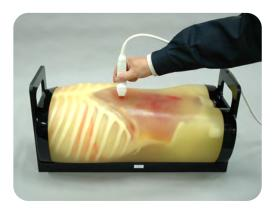
The phantom can be scanned with actual ultrasound devices.
