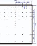
Nylon strings targets for image distortion assessment, axial resolution and angular resolution.
